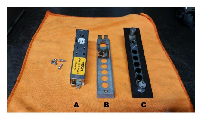
2. With the lid upside down, place the part C into the lid's slot from underneath, as pictured.
