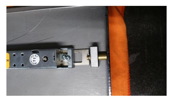
5. Clamp bolt guide block into place and check the lock function. The lock should open and close freely without interference with the lid's front lip or the bolt guide block.
