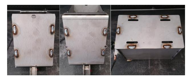
8. Weld the side panels between the tab locations as shown. Avoid welding near the holes in the rear panel where the rear cup holder mounting bolts pass through.
