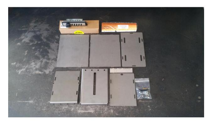
Take note of the orientation of the side panels. There is a relief cut for the spring hinge (circled in red).
