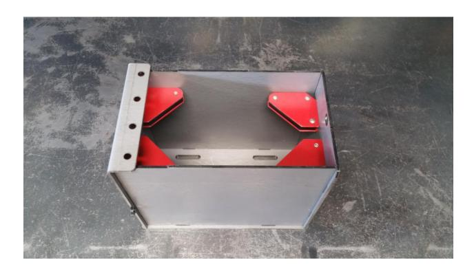
4. Slide the hinge into place in the relief cut, underneath the rear panel's top flange, as pictured.
