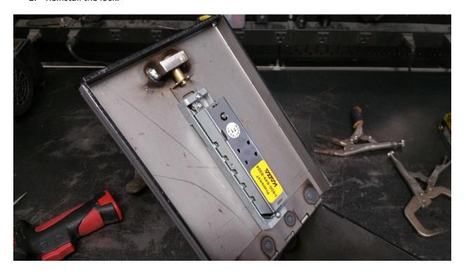
3. The lock chassis should sit flush against the lid. If there is a gap along the red line pictured below, there may be a slight interference between the lock chassis and the hinge leaf (circled in red). If so, slightly radius the rear edge of the chassis with a grinder and reinstall the lock. The lock is sitting properly in this photo.
