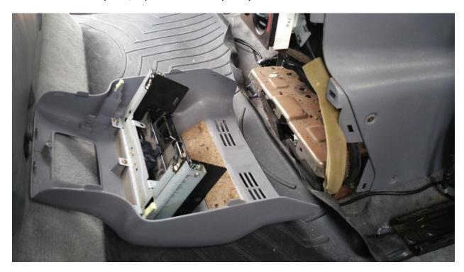
6. Remove the screws holding the rear heater control in place. Rear audio controls or other factory installed options may have different mounting screw locations.
