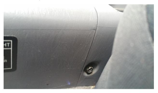
3. Remove the two lower screws, one on either side of the rear portion of the center console. These are hidden by the front seats. Slide the seats forward to gain access.
