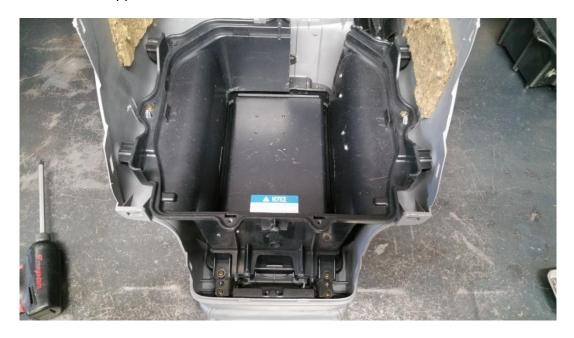
16. Reinstall the center console and console bezel. Reattach the rear panel with the supplied large Phillips screws. Do not overtighten as the rear cup holder bracket can bend. Opening the center armrest and upper console cubby, you should now see this cavity:
