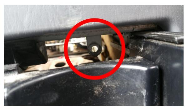
5. Pull the rear panel/cupholder assembly away from the center console.
