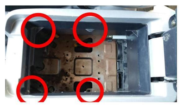
15. Reinstall the upper half of the console liner with twelve screws.
