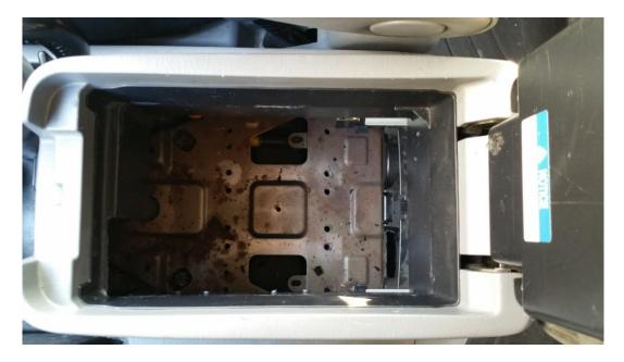
17. Lower the vault into the console cavity. You may find it easier to open the vault and hold onto the lid and front panel to lower the vault into place. Loosely install the screws and washers. Adjust the vault position to the "sweet spot" where the vault door opens and closes without rubbing on the console liner, and where the rear cup holders are properly functioning. Tighten the four screws.
