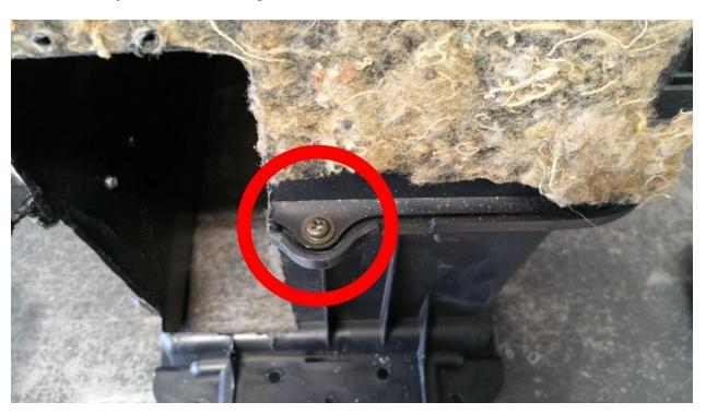
• Two screws underneath the lip (flip entire console right-side up for access)
