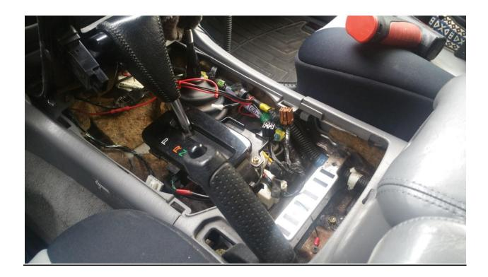
2. Remove the two screws on either side of the front portion of the center console. These are hidden by the front seats. Slide the seats rearward to gain access. A right angle screwdriver may be needed.
