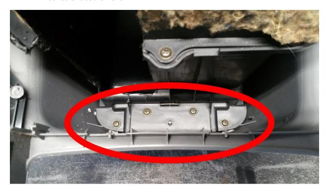
• Two screws, one on either side of the console liner
